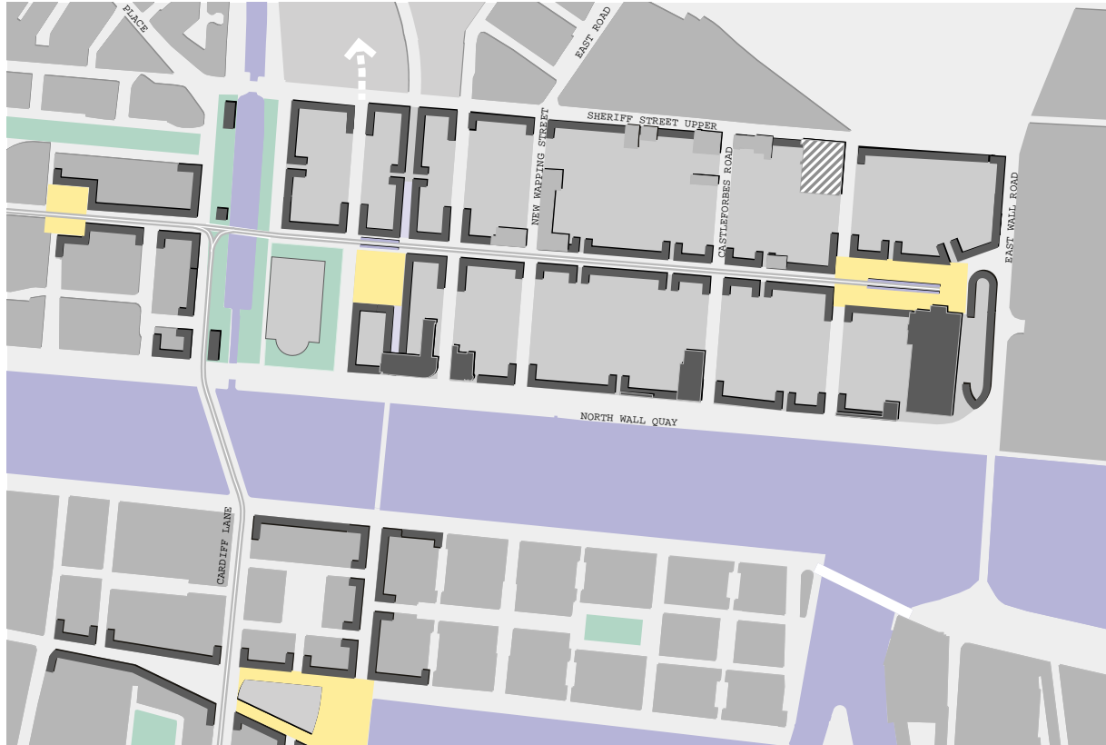
Diagram 12 Main urban structure showing the central spine, Liffey frontage development and north-south pedestrian spine on the line of the new pedestrian bridge to Grand Canal Dock. (Modification No. 4)
